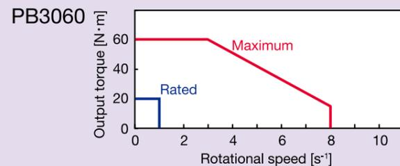
\*Speed – Torque curve is typical value measured in 200 [VAC] (PB3060 : 220 [VAC]).
