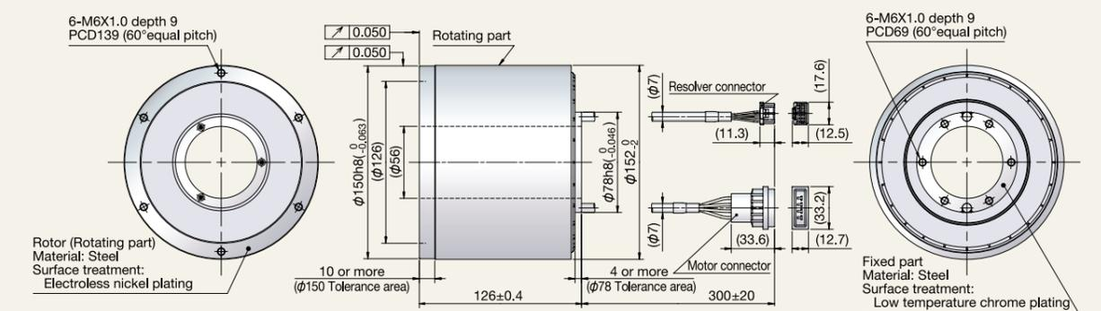
1. The bend radius of the motor cable lead (φ7) and the resolver cable lead (φ7) should be R30 [mm] or more.
